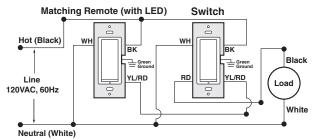
NOTE: The switch must be installed in a wall box that has a Load connection. The matching remote **must** be installed in a wall box with a Line Hot connection and a Neutral connection. A Neutral wire to the matching remote needs to be added as shown.
